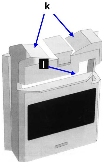
The adapter for sharpening knives and scissors is suitable for sharpening all household knives and scissors with straight blades. Serrated or wavy blades can not be processed.
